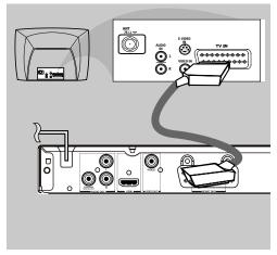
Use the scart cable to connect the DVD SCART OUT to the corresponding scart input socket on the TV (cable not supplied).
