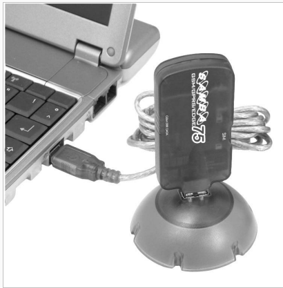
Figure 7.a: Connect USB connector of SAMBA 75 to the USB serial port of PC. (Note that, the SAMBA-USB-Kit is not a part of modem SAMBA 75).
