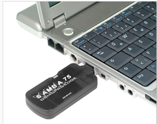
Figure 7.b: Connect USB connector of SAMBA 75 to directly to the USB serial port of PC.
