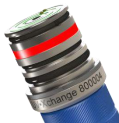
Close-up of stem engraving showing serial number. From top to bottom: stabilizing o-ring, sealing o-ring, locking o-ring.
