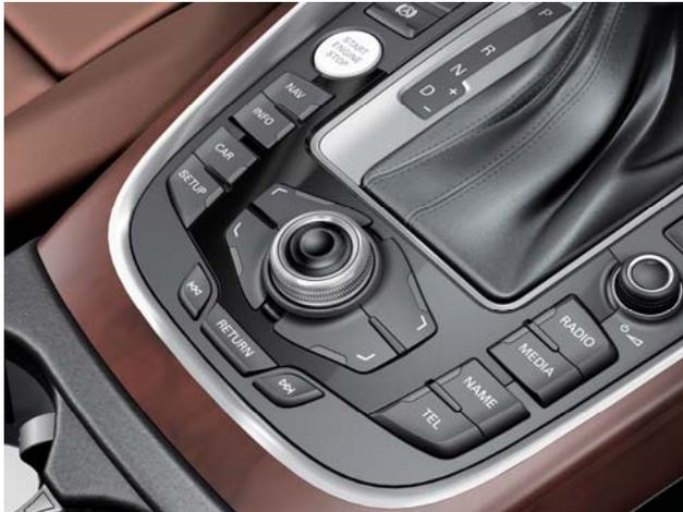
Figure 2: MMI control unit with integrated joystick
