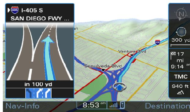
Figure 8: 3D motorway exit display with lane-level guidance
