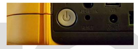
**Step 1:** Start by plugging the unit in to the PoE injector to begin charging the unit. You can use the unit while it is being charged. Connect the PoE injector with an Ethernet cable to the RJ 45 port labeled 'Charge' (it is green in color).
