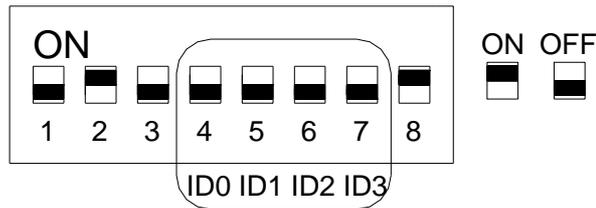
The setting shown above sets the device SCSI ID to "0."
