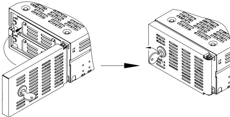
10. Mount the **Mirror Drive** in the host computer. Firmly connect the SCSI cable and 4-pin internal power cable.
