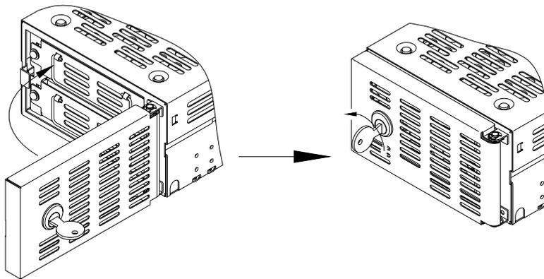
9. In seconds, data rebuilding will start, while the drive status indicator for the replaced drive unit lights green. The drive status indicator for the correctly functioning drive unit will not light. The access indicator will flash orange.
