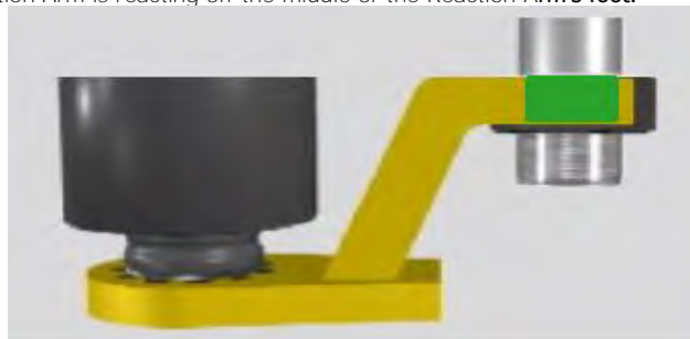
Figure 3.2.4-1: Correct Reaction Point
