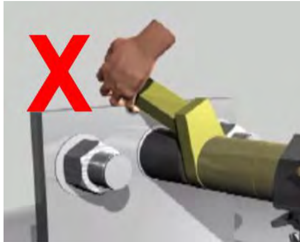
Figure 3.2.1-2: Incorrect Placement of Hand/Body Parts During Operation
