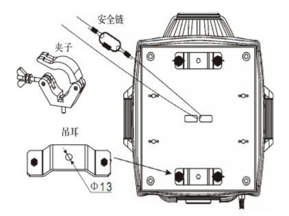
The strand wire is usually used in the shelf for the safety,the strand wire should stand ten times weith than the machine.you should ues the stand wire which has safety lock pins,the strand wire pass through the hole at the bottom,then tie it to the fixity.then tighten it.
