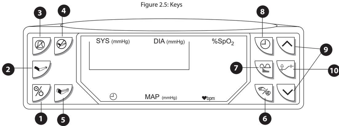
**WARNING!** Verify that all LEDs (light emitting diodes) on the display light up upon startup of the device.
