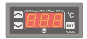
Cool/Freeze thermostat with a temperature sensor, two defrost sensors, a day/night digital input, relays for defrost-1, defrost-2, fan, cool and alarm.
