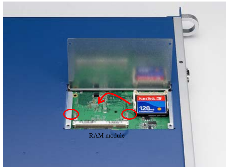
Figure 2-5: Install RAM module
