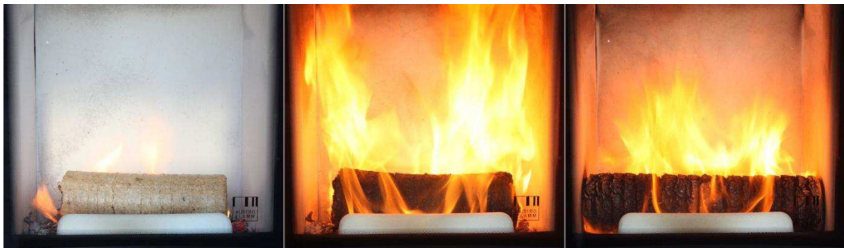
Figure 7: Swelling of wood briquettes in the firebox: The briquette is finally stuck between the walls of the firebox and loses contact to the embers. Therefore: break longer briquettes before charging (source: TFZ)
