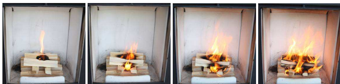
Figure 16: Ignition phase and start of wood combustion (source: TFZ)
