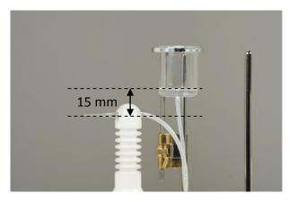
**12.** With the HV Adj. knob turned to zero, **turn on the switch**. While watching closely to the tip of the electrospinning needle; **raise the voltage** until the **Taylor cone** appears this is normally visible with the naked eye. Normally only a very slight increase in voltage will initiate the spinning process.
