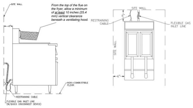
Figure 2. Fryer Site Installation Requirements
