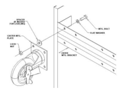
Figure 4. Typical Caster Installation
