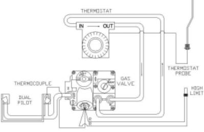
Figure 1. Fryer Model 14GS Wiring Diagram
