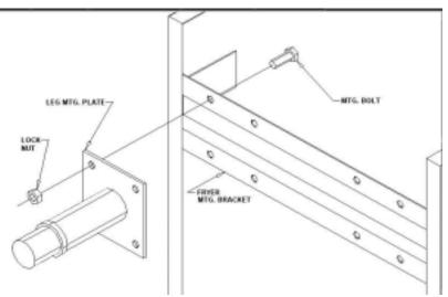
Figure 3. Typical Leg Installation
