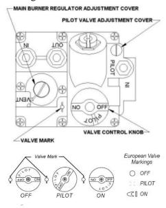
Figure 6. Gas Control Valve & Knob Positions
