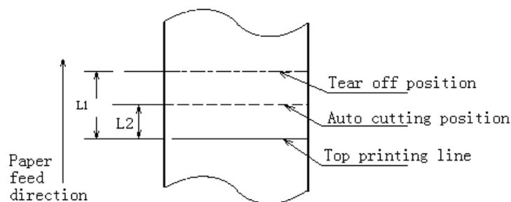
L1 (Distance between Top printing line and Tear off position): about 28mm
