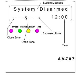
Most of the accessible functions with the LCD Keypad are similar to those of the AV-701 (seven segments keypad).
