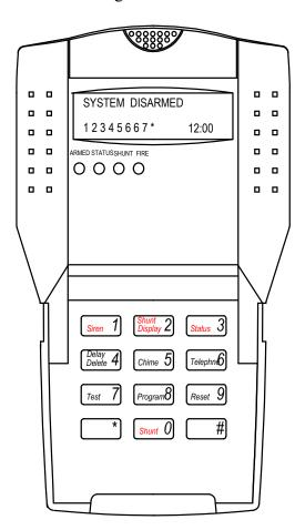
entered (the 'location'), the upper line is cleared, the blinking cursor moves to the beginning of the line, three Rightmost LEDs start blinking indicating that data is expected (in this case the new User Code).
