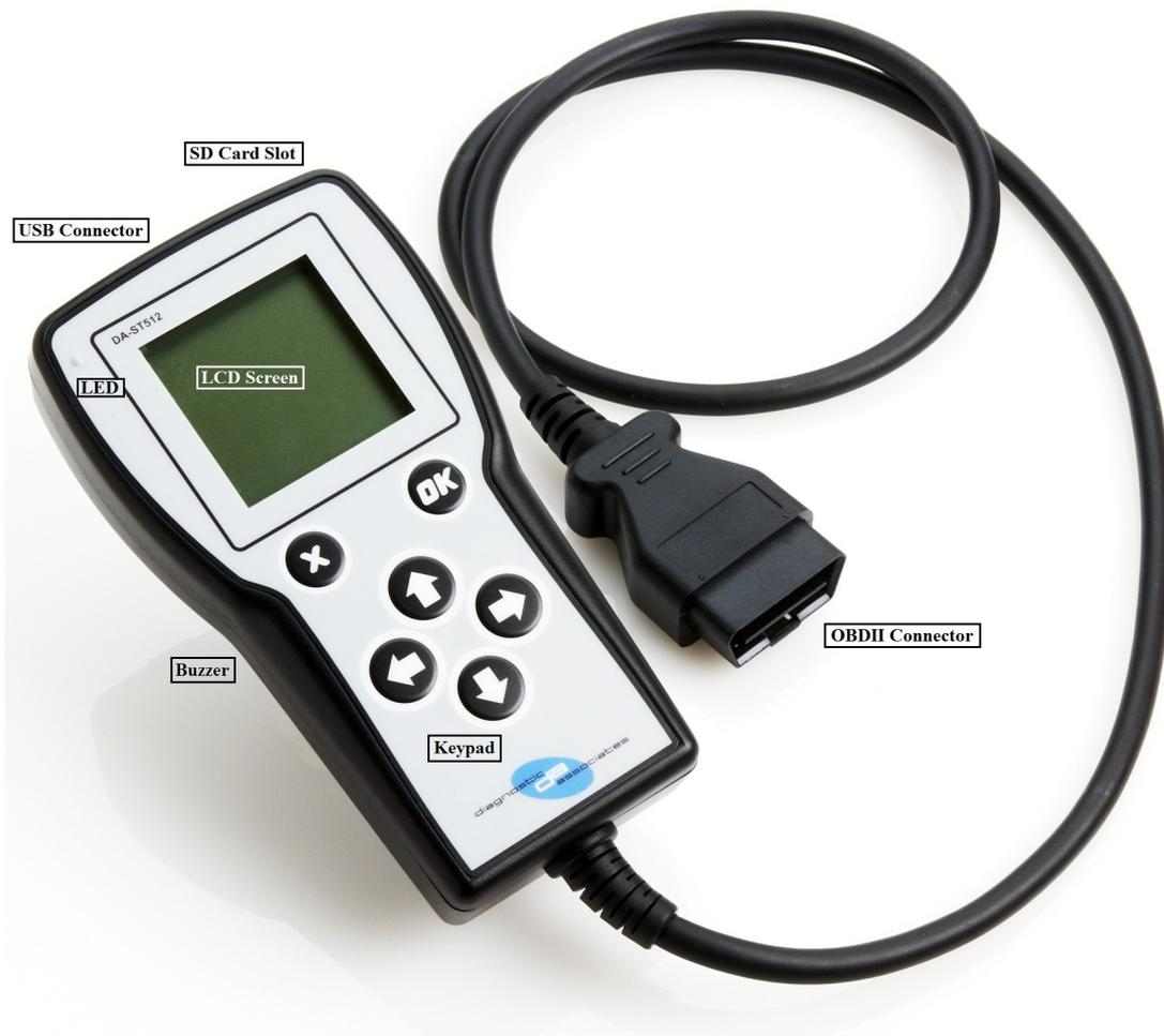
There are seven main parts to the device and these are shown on the picture above.
