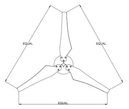
*Fit the Rotor Blade Assembly-* The assembled and balanced rotor blades can now be fitted to the *Chinook 200* chassis. This is done by placing the rotor hub plate against the bearing house on the turbine. In the hardware kit you will find 4 ea 5mm X 12 hex head screws. NOTE, you will have 3 ea 5mm X 14 hex head screws that are LONGER for use on the Nose cone. Ensure that all 4 screws are securely tightened and that the rotor blades are mounted with the flat side of the blades facing forward.
