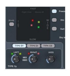
There are four bucket-brigade emulations, two for the left and two for the right channel. Each delay is modulated in frequency and range, according to the position of the lights.
