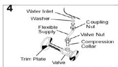
Connect the cold water line to the tank with your straight or angle stop. Place the washer, then the plastic nut on the tank end of the connecting pipe and bend the pipe to fit into the inlet hole on the water regulator. Tighten all coupling nuts securely. **DO NOT USE PLUMBERS PUTTY!**
