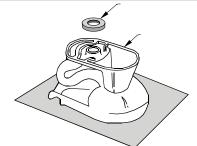
Clean the immediate floor area thoroughly. Insert new toilet bolts in the slotted flange, bolt heads down. The toilet bowl should be placed upside down, on soft material to prevent scratching. Place the slightly warmed wax ring in the circular recess in the base of the bowl. **NOTE:** It is recommended that a wax setting ring with flange be used.
