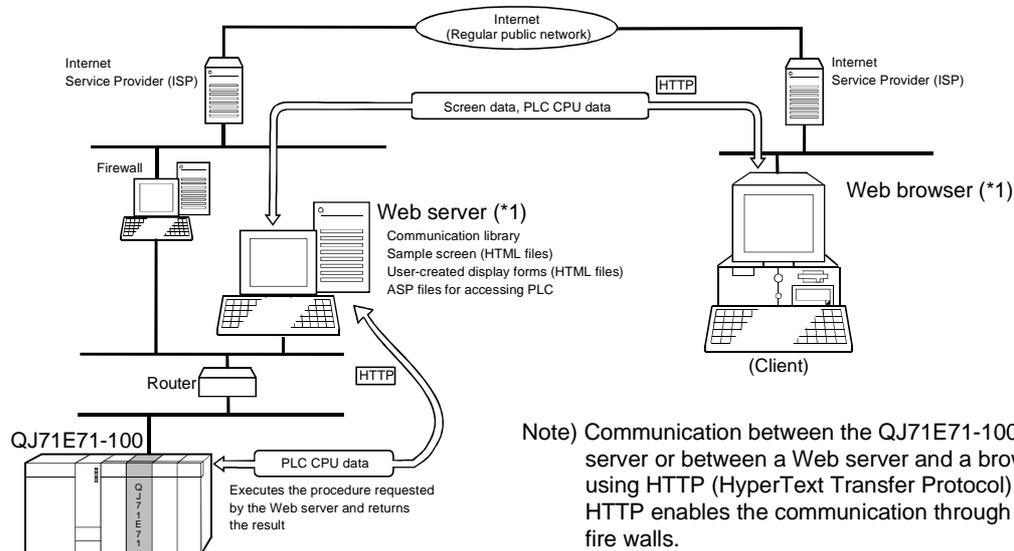
Note) Communication between the QJ71E71-100 and a Web server or between a Web server and a browser is performed using HTTP (HyperText Transfer Protocol). HTTP enables the communication through proxy servers and fire walls.
