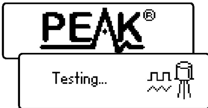
For the first analysis (after the unit has been switched off) the tests are performed while displaying the Peak logo.
