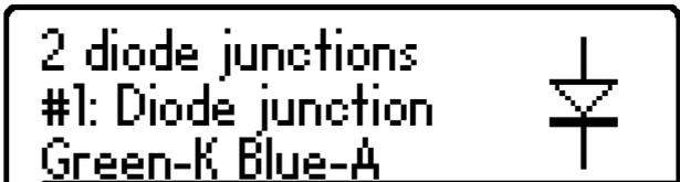
The details for the first diode are then displayed (Diode #1). In this example, the Green test clip is on the Cathode of diode #1 and the Blue test clip is on the Anode.
