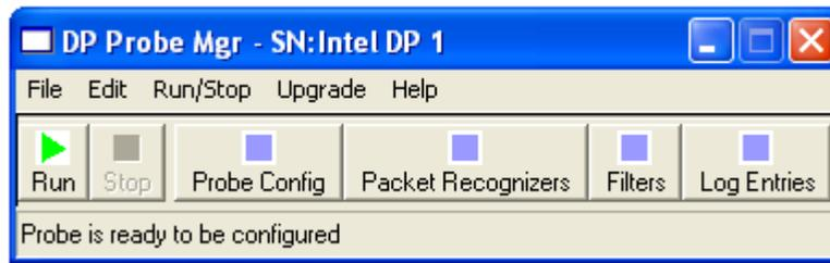
The user configures and controls the preprocessor from the main form. The form is composed of a menu bar, a tool bar and a status message bar. The menu bar provides options that allow the user to configure and run the probe. The tool bar provides options to configure the preprocessor and the status bar displays the probes current status and/or any errors that may have been encountered. Error messages displayed in the status bar are also logged in the Log Form if logging is enabled.
