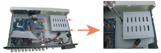
STEP 2:Remove HDD Bracket
