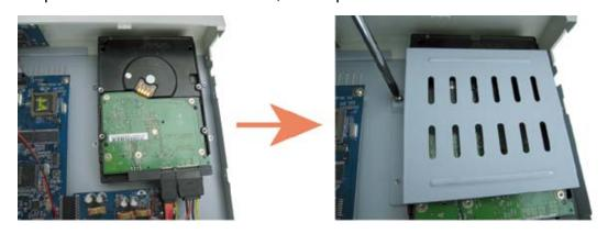
STEP4: Put the HDD and replace the bracket back
