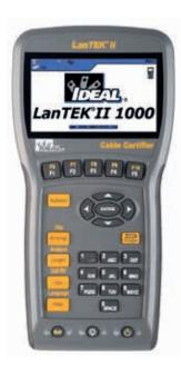
LanTEK II is used for the certification of twisted pair, coax and fiber optic data cable to ensure full compliance with TIA-568 performance standards. Certification reports may be used to obtain warranties from connector and cabling system manufacturers.
