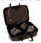
The FiberTEK® FDX option allows standards compliant fiber optic certification capability to be added to any LanTEK® II series certifier.
