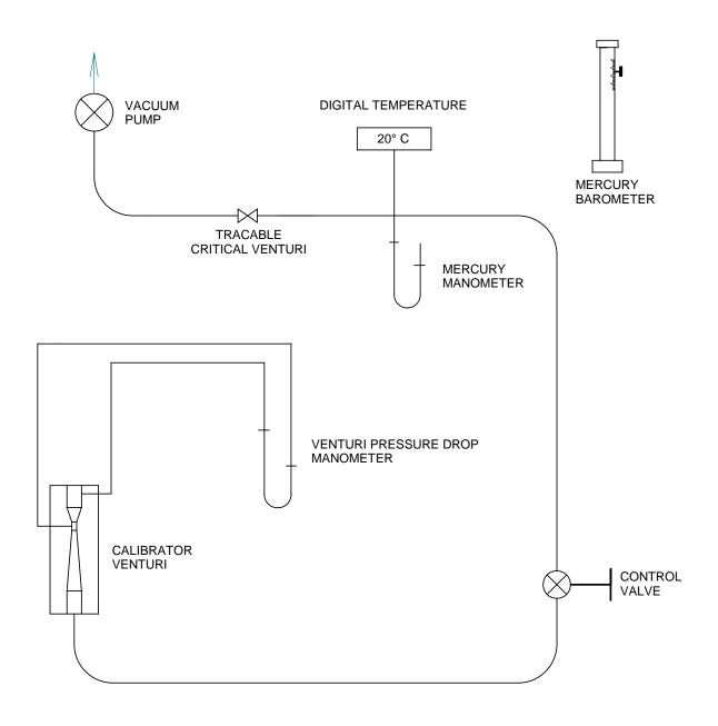
Figure A1- Schematic Diagram of Calibration Setup
