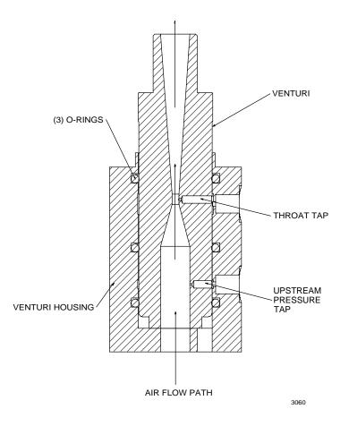
Figure 3 – Sectional View of Measuring Head
