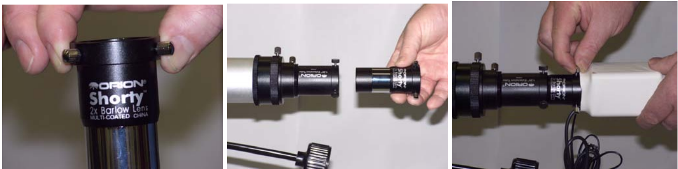
Figure 8: Inserting the Shorty 2X Magnification Lens
