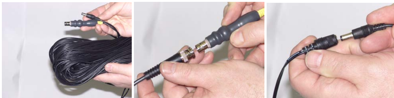
Figure 10: Connect Power and Video on the Camera Side
