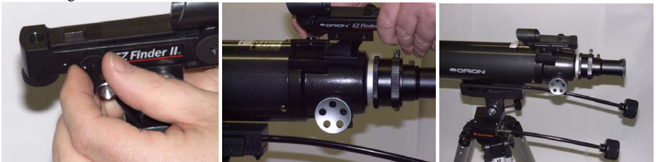
Figure 5: Attaching the Red Dot Viewfinder
