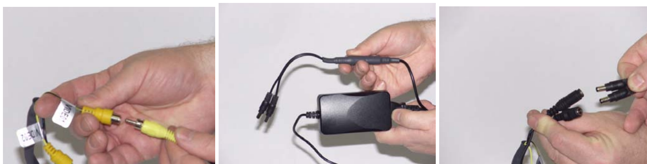
Figure 12: Connect Power and Video to LCD Side
