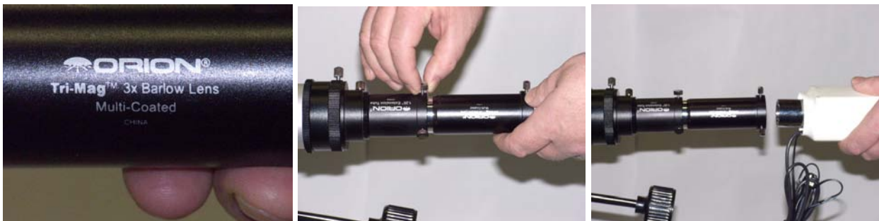
Figure 9: Inserting the Tri-Mag 3X Magnification Lens
