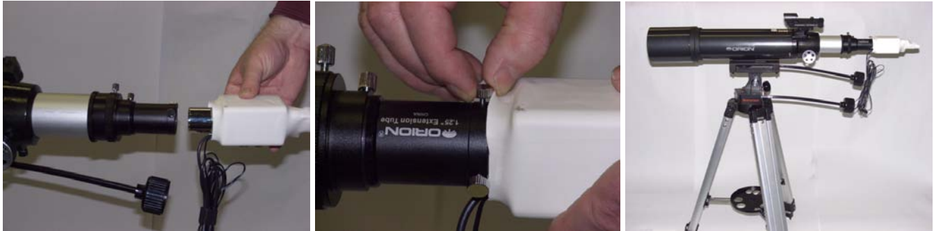
Figure 7: Attach the camera
