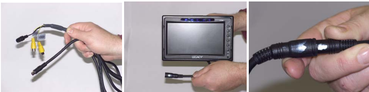
Figure 11: Connect Integrated Cable to LCD Unit
