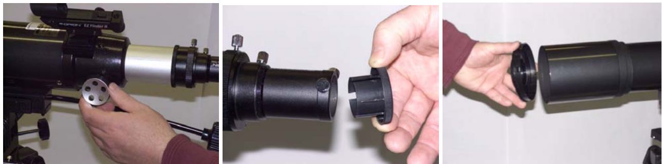
Figure 6: Pull out focus and remove lens caps on both ends
