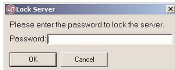
Enter the lock code, and Click "OK." If successful, the status section should now display a locked status:
