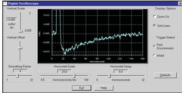
Figure 42 Undercompensated Pole/Zero Using a Nal(Tl) Detector
