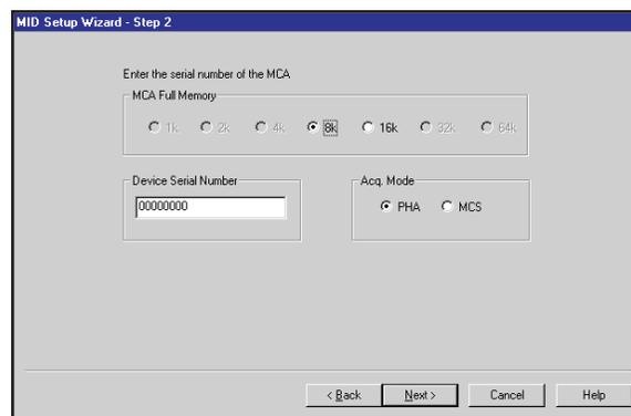
Figure 9 Defining the Full Memory and Device Serial Number for USB Operation
