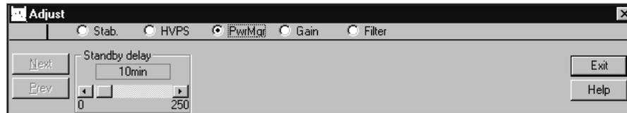
Figure 26 Adjust Screen's Power Management Settings
