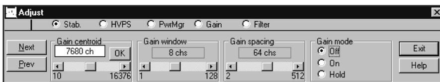
Figure 22 Adjust Screen's Stabilizer Settings
