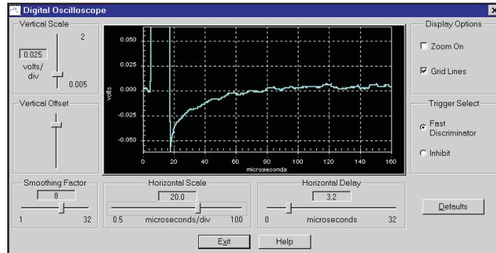
Figure 40 Undercompensation Pole/Zero
