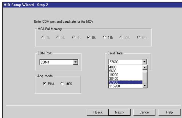
Figure 11 Setting the Baud Rate for RS-232 Operation
