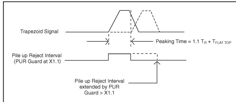
Figure 35 PUR Reject Interval
