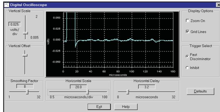
Figure 38 Correct Pole/Zero Compensation
