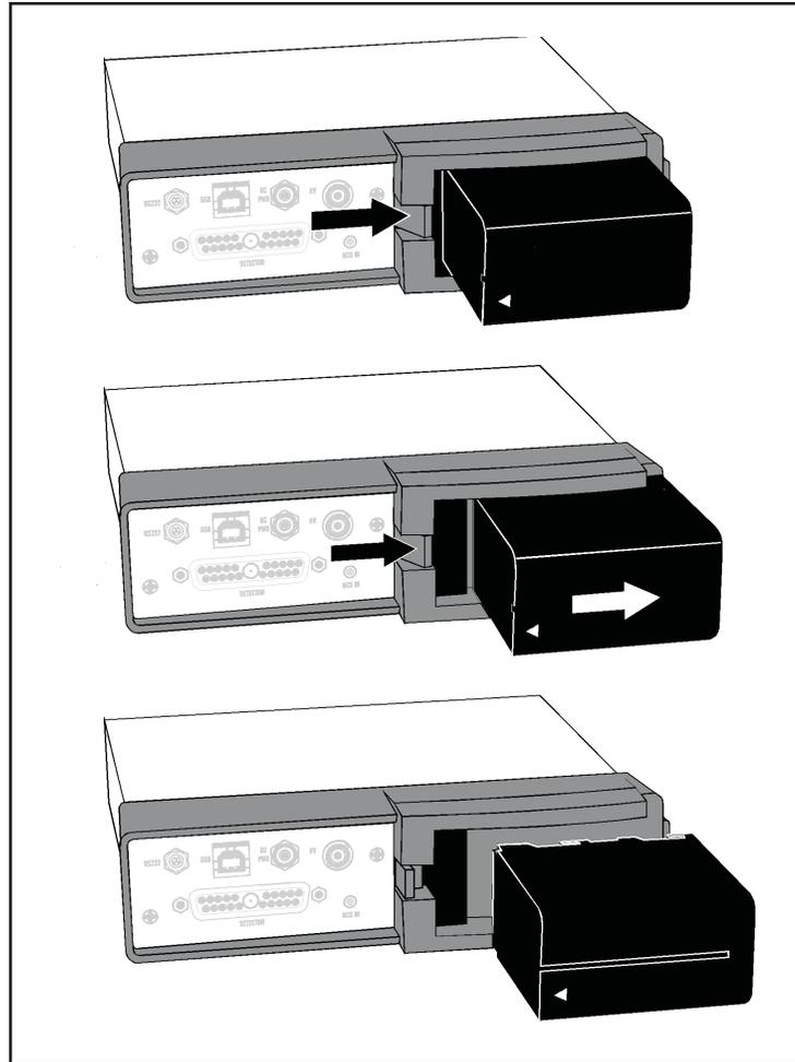
Figure 5 Removing the Battery
