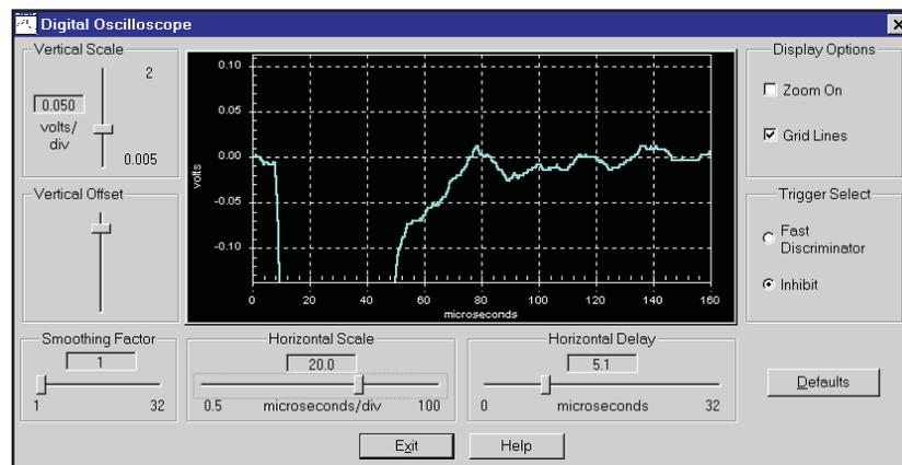
Figure 45 Digital Oscilloscope Waveform Showing Trapezoid Filter Reset Period
