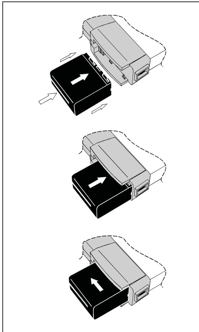
Figure 4 Attaching the Battery
