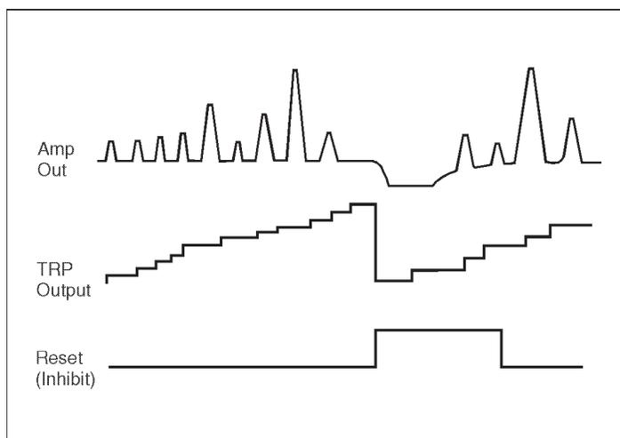
Figure 44 Monitor Output, TRP Output, TRP Inhibit
