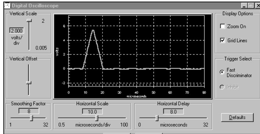
Figure 31 Digital Oscilloscope Screen Showing Detector Trapezoid Waveform
