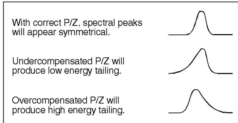
Figure 37 Pole/Zero Compensation - Examples
