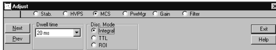
Figure 25 Adjust Screen's MCS Setting
