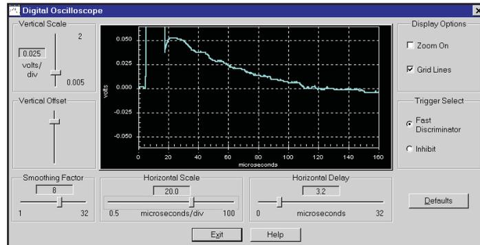
Figure 39 Overcompensated Pole/Zero
