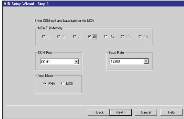
Figure 10 Defining the MCA Full Memory, COM Port and Baud Rate for RS-232
