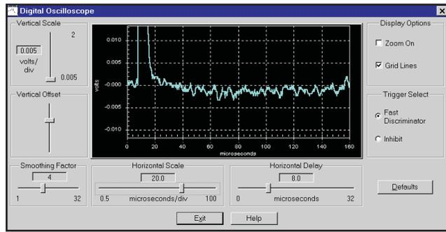
Figure 41 Correct Pole/Zero Using a Nal(Tl) Detector
