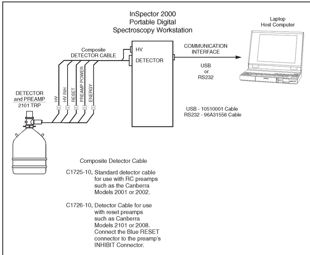
Figure 32 Typical Gamma Spectroscopy
