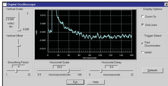
Figure 43 Overcompensated Pole/Zero Using a Nal(Tl) Detector
