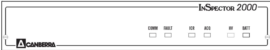
Figure 1 InSpector 2000 Front Panel
