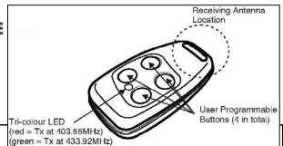
The following procedure explains how to learn existing transmitters into your SENTRY learning remote control. For best results the transmitter to be learnt MUST be placed in close proximity to the receiving antenna, which is located alongside the keyring side of the TX4 Dual.
