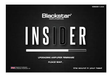
Please do not disconnect or switch off your amplifier whilst the firmware is being updated; as this may result in your amplifier becoming non-functional. If this occurs the TAP indicator on the front panel of your ID:Series amplifier will flash in isolation. Please connect it to your computer via USB and run the Blackstar INSIDER software. The problem will be detected and the firmware will be restored to your amplifier.
