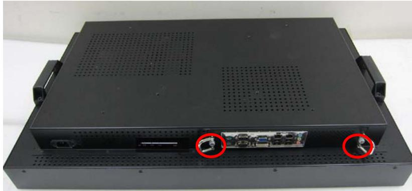
**Step 3** Pull out the engine box via the rings as marked.
