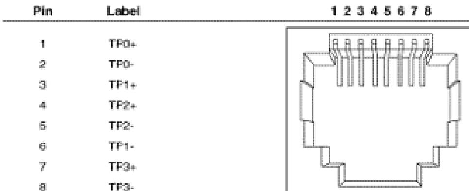
■ **10/100/1000Base-TX Cable Schematic**
