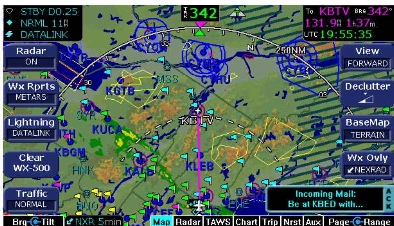
Figure 13.8 Incoming Message Alert
