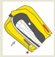
Fold the lung up. First fold the side where the re-arming mechanism is found. Remember to close the Velcro opening. Fold in layers as shown\*. The pull card is to be fed out through the Velcro.
