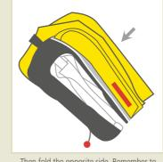
Then fold the opposite side. Remember to close the Velcro opening. Ensure that the nozzle is easily accessible. Attach the grab loop over the nozzle.
