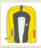
The lifejacket is flattened and is prepared for packing.
