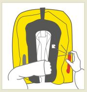
Remove all the air by pressing the valve cap on the nozzle and applying pressure to the lung.
