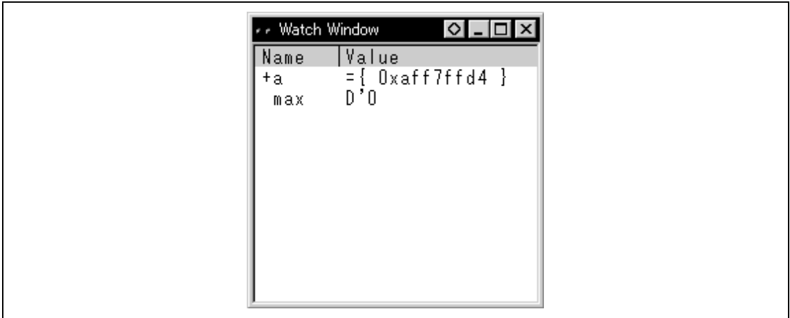
Figure 3.23 [Watch Window] Window (Displaying the Variable)
