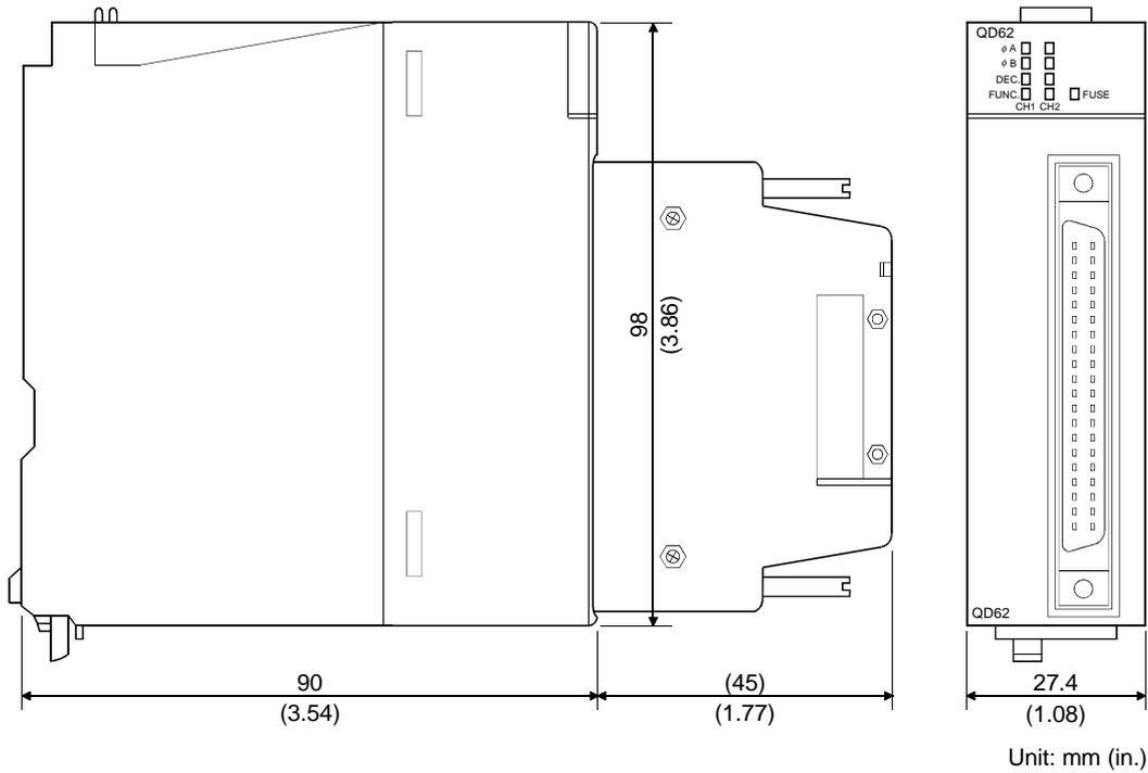
A value in parentheses shows the reference measurement when the A6CON1 is installed.
