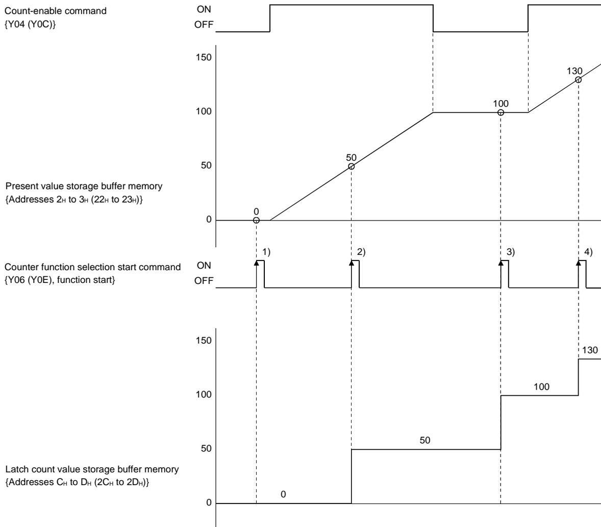
When the counter function selection start command {Y06 (Y0E), function start input} rises at points indicated by 1) to 4) in the figure above, the present counter value is stored in the latch count value storage buffer memory {addresses CH to DH (2CH to 2DH)}. The latch counter function is executed regardless of whether the count enable command {Y04 (Y0C)} turns ON/OFF.
