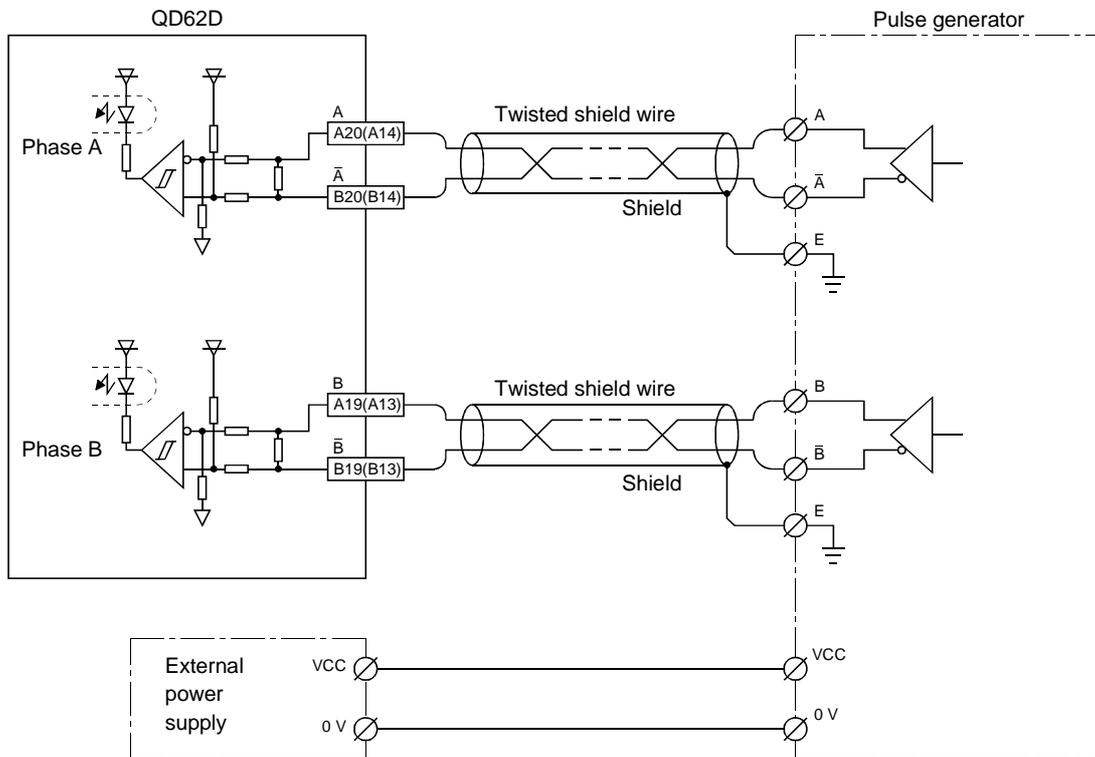
The number inside the ( ) indicates the terminal number for channel 2.
