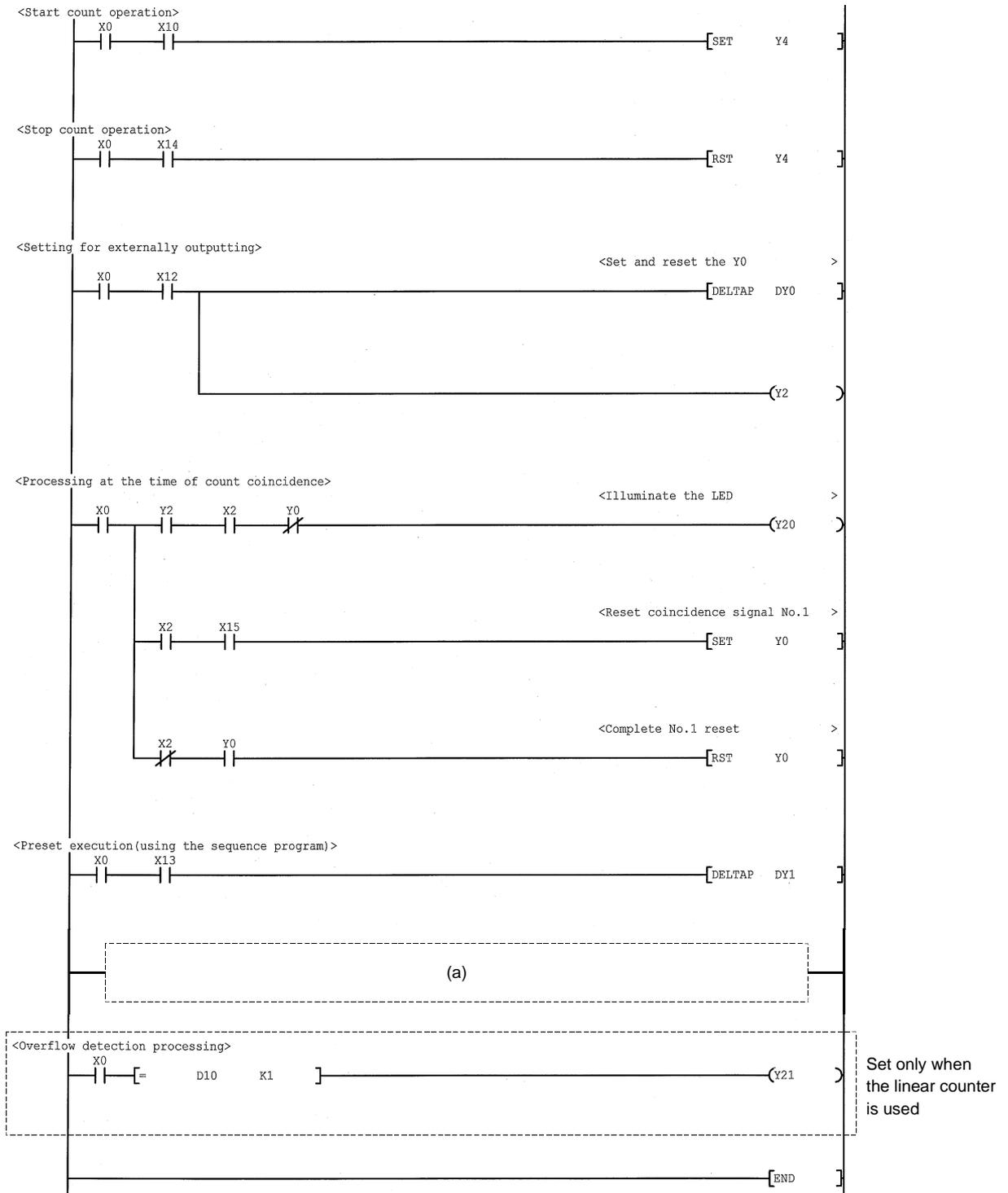
(a) When using the functions listed below, the following programs are inserted.
