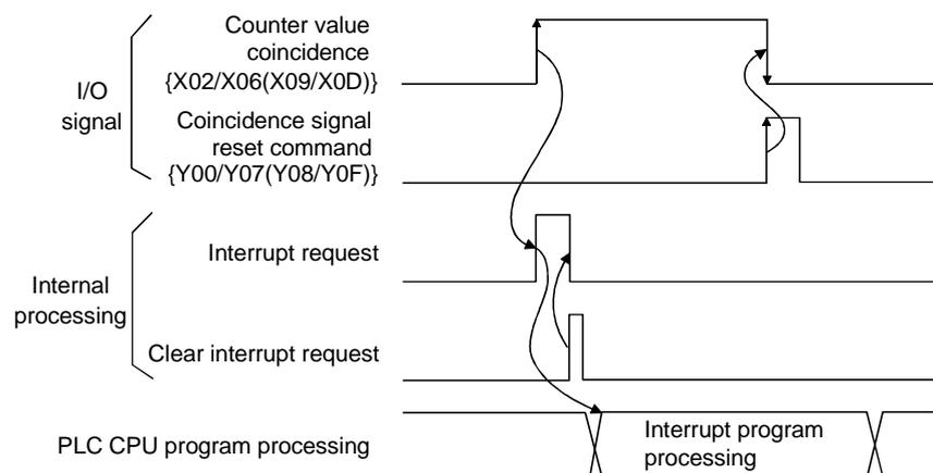
(b) Assignment of the interruption factors (SI) and the interrupt pointers for PLC CPU are set by selecting "PLC parameter" - "PLC system" - "Intelligent function module setting" - "Interrupt pointer settings".
