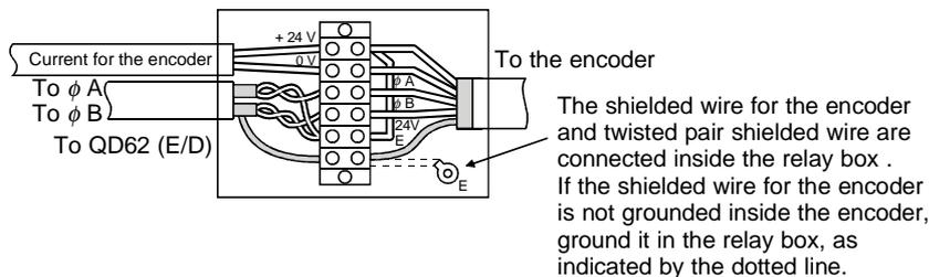
4.4.2 Wiring example of a module and a pulse generator
