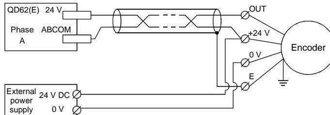
[Incorrect wiring example]
