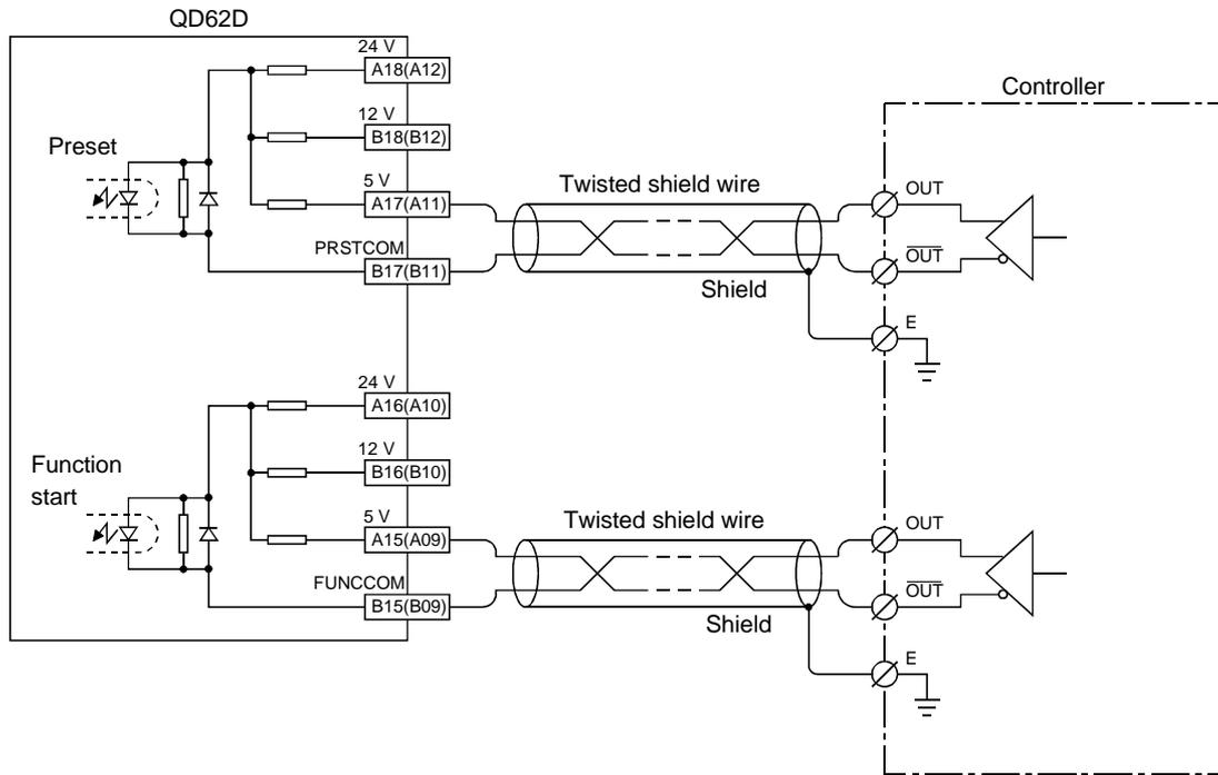
The number inside the ( ) indicates the terminal number for channel 2.
