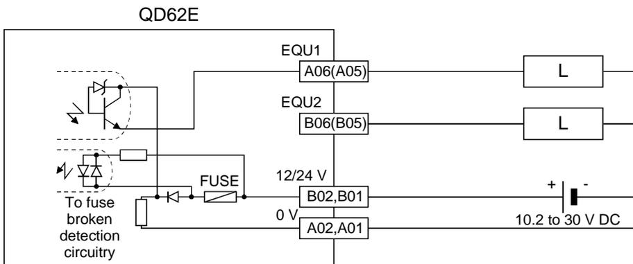
The number inside the ( ) indicates the terminal number for channel 2.
