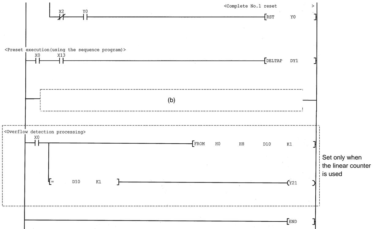
(a) When using the sampling counter function and the periodic pulse counter function, the following programs are inserted
