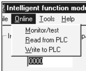
[Monitor/test] : Starts the select monitor/test module screen.
