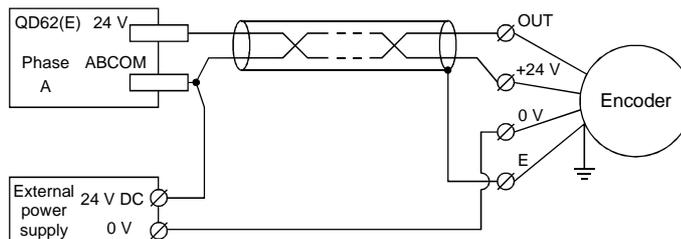
The current flows through the twisted pair cables in the same direction, so there is no cancelling effect. This makes it more prone to electromagnetic induction.
