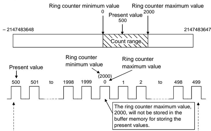
(a) The ring counter will operate as follows when the "present value < ring counter minimum value" or "ring counter maximum value < present value".
