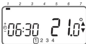
b. To adjust the period start time use the (⏪) (+) or (⏩) (-) buttons, the 'OK?' indicator will be displayed to confirm the change. Holding the button down will change the time quickly.
