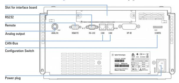
Figure 9 Rear of the Binary Pump
