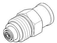
**4** Reinstall the outlet valve and tighten it using a torque wrench (12 Nm).
