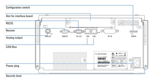
Figure 27 Electrical connections to the binary pump
