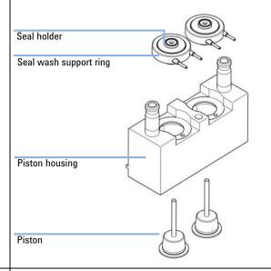
3 Check the piston surface and remove any deposits or layers. Most suitable is polishing of the piston rod with toothpaste. Replace the piston if scratched or if dents are visible.
