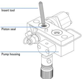
5 Using the plastic side of the insert tool insert the new seals into the pump head and press them firmly in position.
