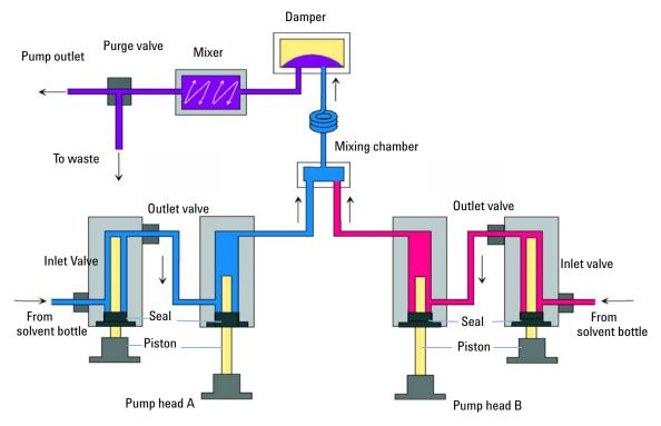
Figure 2 The Hydraulic Path
