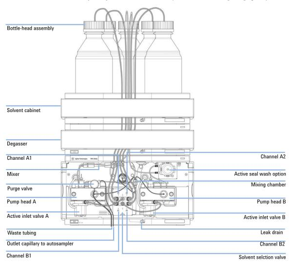
Figure 11 Binary Pump with Solvent Selection Valve
