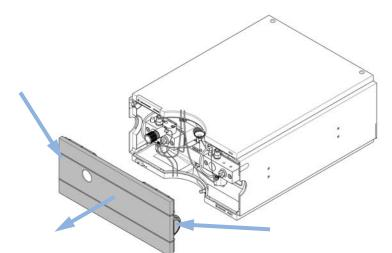
1 Remove the front cover by pressing the snap fasteners on both sides.
