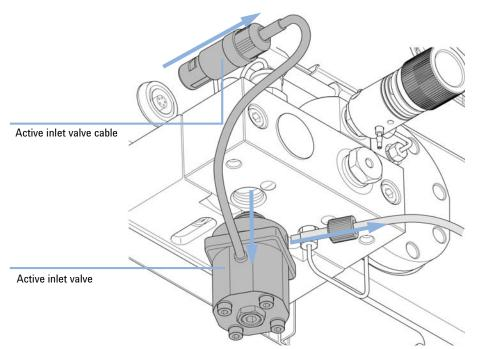
**5** Using a pair of tweezers, remove the valve cartridge from the defective active inlet valve.
