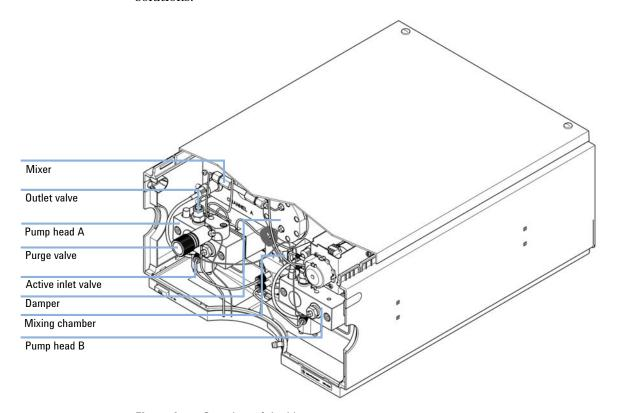
Figure 1 Overview of the binary pump
