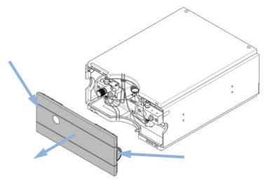
Figure 12 Removing the Front Cover
