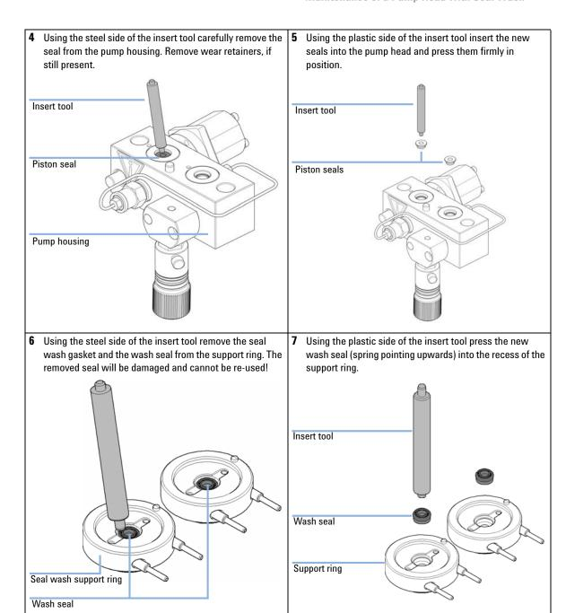
Maintenance of a Pump Head with Seal Wash
