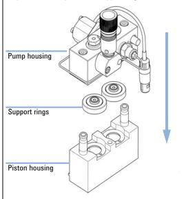
Maintenance of a Pump Head without Seal Wash
