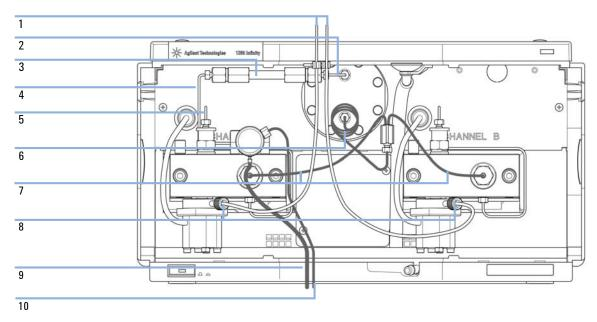
Figure 25 Hydraulic Path without Solvent Selection Valve
