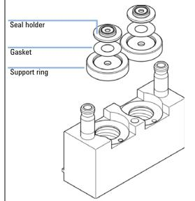
**7** Reassemble the pump head assembly. Note the correct position of the pin on the support ring.
