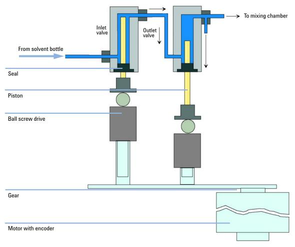
Figure 3 Principle of Pump Unit
