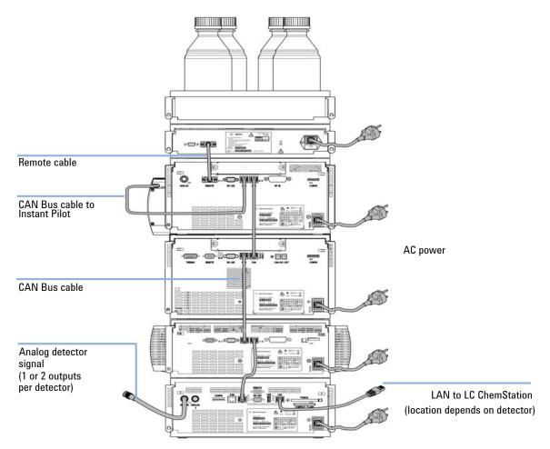
Figure 5 Recommended Stack Configuration for 1260 Infinity (Rear View)
