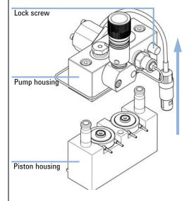
2 Remove the seal holder and the seal wash support rings from the piston housing. Remove the seal holder from the support ring assembly.
