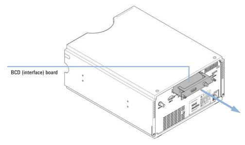
Figure 16 Exchanging the Interface Board
