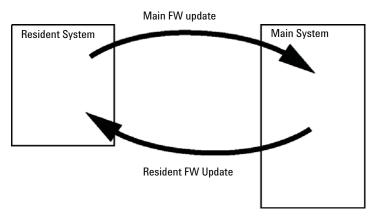
Figure 26 Firmware Update Mechanism
