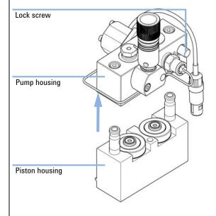
2 Remove the support rings from the piston housing and lift the housing away from the pistons.
