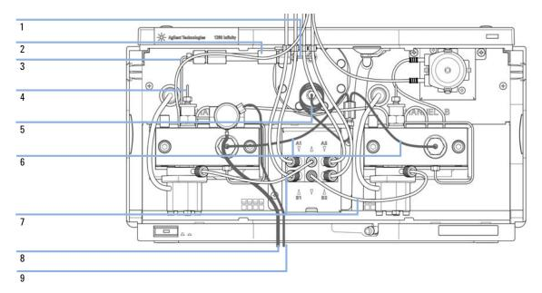
Figure 24 Hydraulic path with solvent selection valve and active seal wash option
