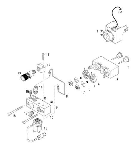
Figure 18 Pump head assembly with seal wash option
