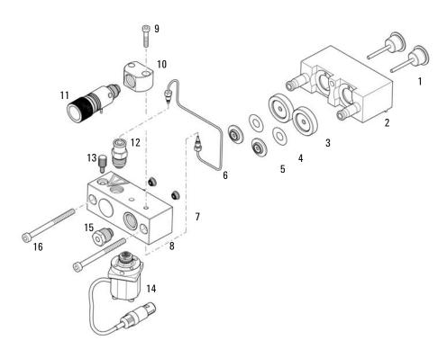
Figure 17 Pump Head Assembly Without Seal Wash
