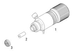
Figure 20 Purge Valve Assembly
