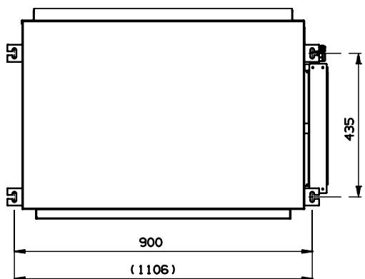
**EG** Mark on the ceiling the holes for the hanging rods, verify the distance of the centres. The value included in the brackets is referred to the model UR18-22X.
