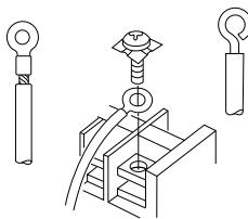
**EG** Predispose the terminals of the wire to connect to the terminal strip and connect them. (See electric wiring to connect).
