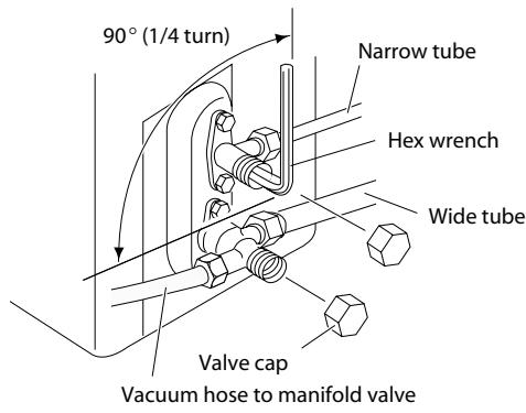
**EG** Turn the service valves stem in counterclockwise to fully open the valves. At this point vacuum pump flexible hose can be disconnected. Replace bonnet and flare nut, tighten them to 200 kg/cm with a torque wrench.
