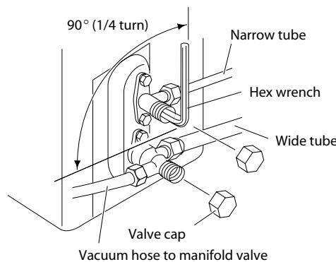
**EG** With vacuum pump still running close the low pressure knob on valve manifold. Then stop vacuum pump. Using an hexagonal key open the service valve on small tube, then close it after 10 seconds. Check tightness of all joints using liquid soap.
