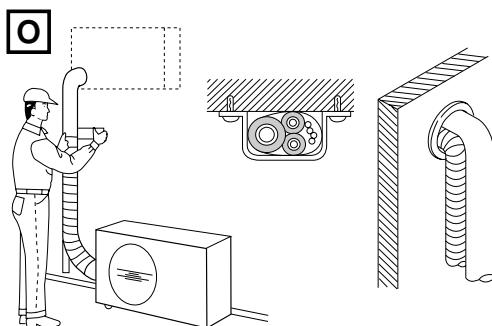
**O** **EG** Complete insulation of refrigerant tubes; wrap with insulation tape. Fix and support tubes with brackets. Seal hole in the wall, if necessary.
