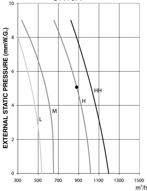
**EG** ● **H:** Standard supplied unit. Available fan speeds: Low-Middle-High (L - M - H). Max. static pressure: about 5 mm
