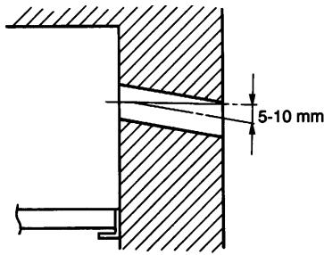
**EG** Drill a 80 mm diameter hole, for the passage of refrigeration pipework, condensate pipework and electrical cable. Insert a PVC pipe in the wall.
