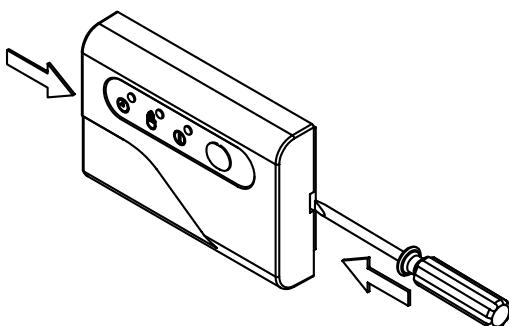
**E** Slot a screwdriver by the 2 slits on the cover sides, and separate the cover from the base.
