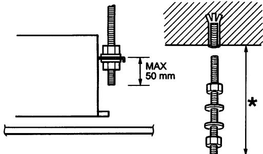
**EG** Use rawl plug suitable to the ceiling consistence and four M10 threaded bars of suitable lenght (not supplied).
