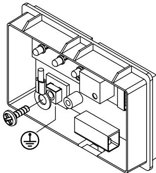
**EG** Perform the earth connection with the terminal on the base, as provided. Complete earth connection and fasten the other end of the cable to the earth terminal in the electric panel.
