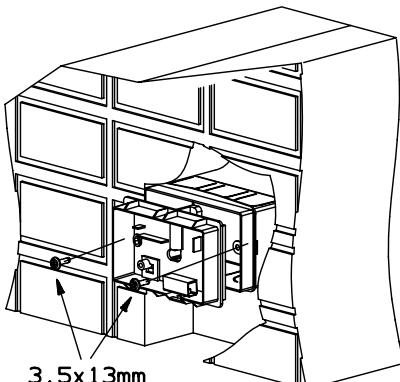
**E** If allowed by the local electric-power standards, standard electric-component boxes can be used for assembling the receiver.
