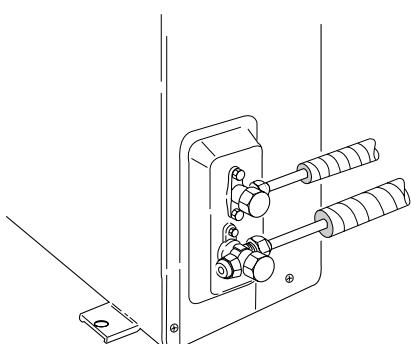
**EG** Remove the valve manifold. At that time, PUMP DOWN has been completed and all refrigerant gas will have been collected in the outdoor unit.
