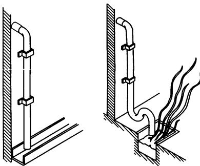
**EG** Convoy the condensate to the outside with a positive slope, from a trap at the end if necessary.
