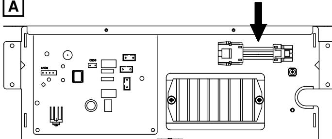
**E** Open the cover of the electrical junction box. Take out the booster cable clamped in the box.
