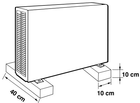
**EG** Provide a solid base for outdoor unit raised from the ground level. Fix unit to base using 4 anchor bolts.
