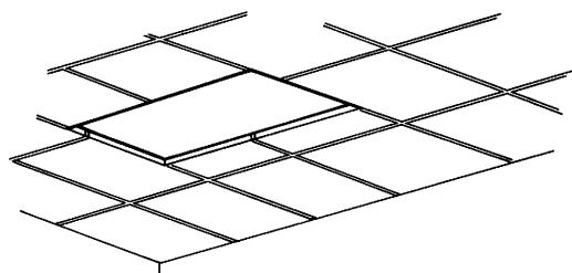
**EG** Find the space for the installation of the return air grille and mark the opening to do. Cut the falseceiling.
