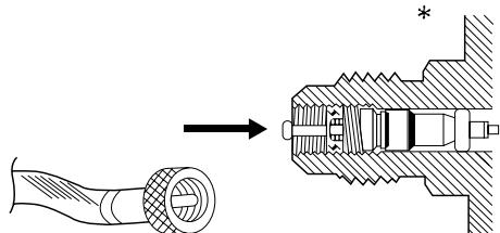
**EG** The service port on the wide tube service valve uses a Schrader core valve to access the refrigerant system. Therefore, be sure to use a hose connector which has a push-pin inside.
