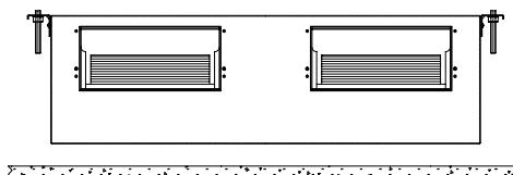
**EG** Secure the unit in position with locknuts and washers, level the unit, keeping the right distance from the falseceiling for the installation of return air grille.
