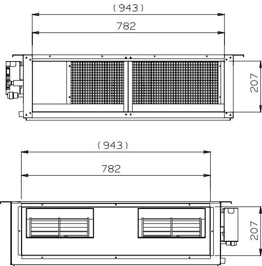
**EG** Rear and front flange for the air intake. The value included in the brackets is referred to the model UR18-22X.
