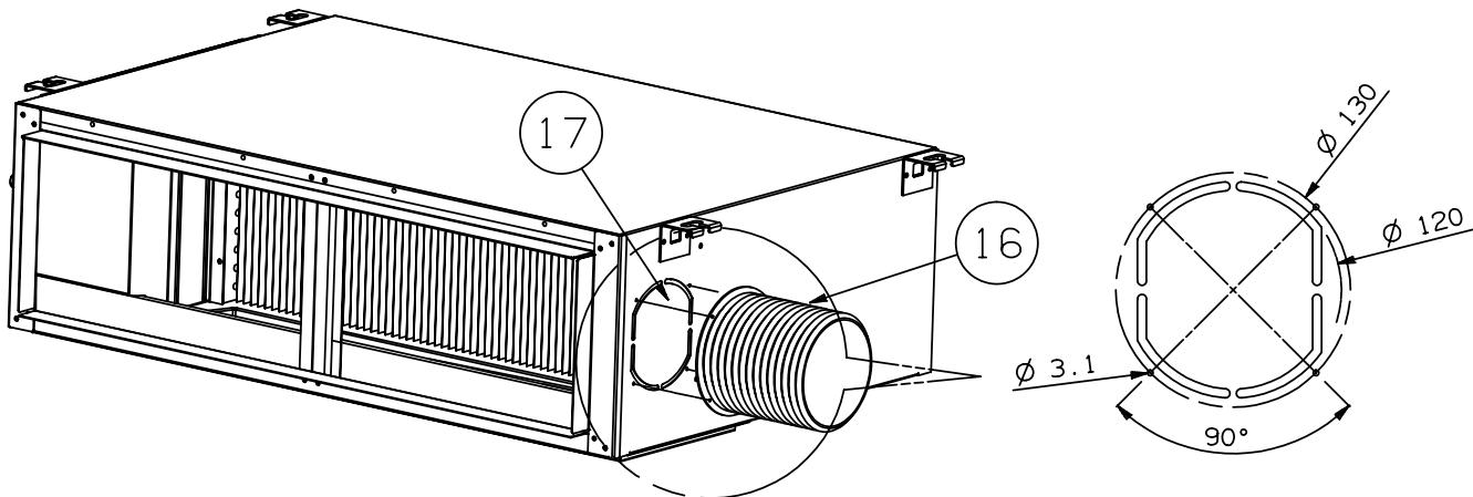
**EQ** There is a duct connection port ⑯ for drawing in fresh air.
