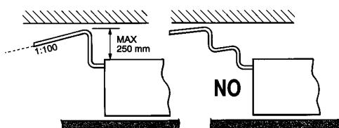
**EG** The unit is supplied of PVC hose from the condensate pump. Maximum pump lift is 250 mm over the unit. Convoy the condensate with a positive slop (min. 1:100) to the outside. The highest point in the condensate pipework should be as close to the unit as possible. This prevents a large volume of water draining back into the unit when it is switched off.
