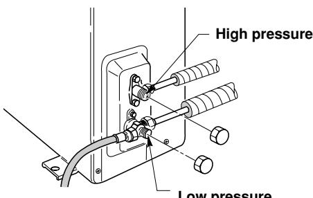
**EG** Remove caps from service valves of both tubes. Then start vacuum pump and let it run for the time indicated in the table (vacuum 10 mm Hg abs.).
