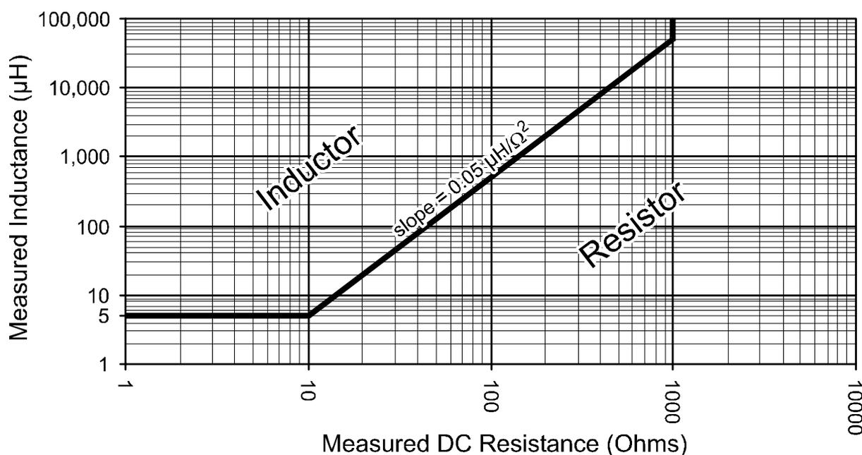
For example, if the inductance of your component is measured at 100µH and it has a DC resistance of 100Ω, then the Atlas LCR will tell you that you have a resistor. If however the resistance was only 10Ω, then the Atlas LCR will tell you that you have an inductor.
