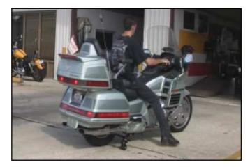
When using the LegUp® LandinGear System, the rider should stop the bike the same way they always did, and basically ignore the LandinGear! We will discuss how to make the wheels deploy later; here we want to talk about techniques when they do!
