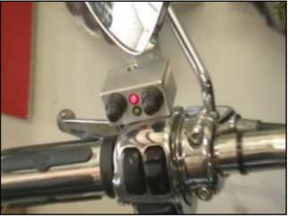
always on. The bottom LED, which is yellow, during normal operation, is on when the legs are up, and it is safe to lower the legs, and it blinks when the legs have been authorized to deploy on the next stop (more about this later!).
