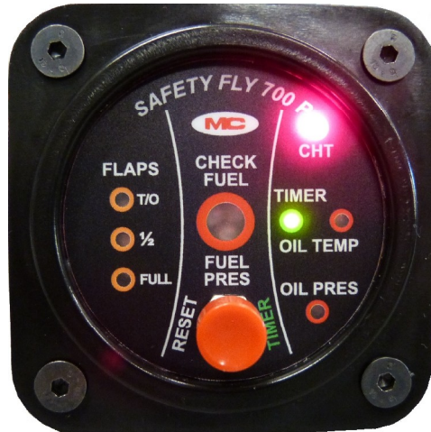
Fig. 7 example of cylinder head temperature alarm
