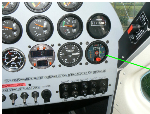
Fig. 1 – SAFETY-FLY 700 P installed on the motor instrument dashboard.
