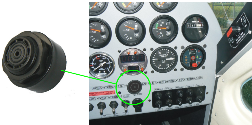
Fig. 4 Buzzer installed on the motor instrument dashboard.
