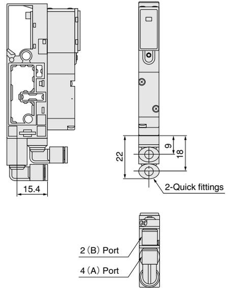
Note: For FMWR090E1, the 2(B) port is plugged, while for FMWR090E1-11, the 4(A) port is plugged ( $\phi$  4: **UP-4**).
