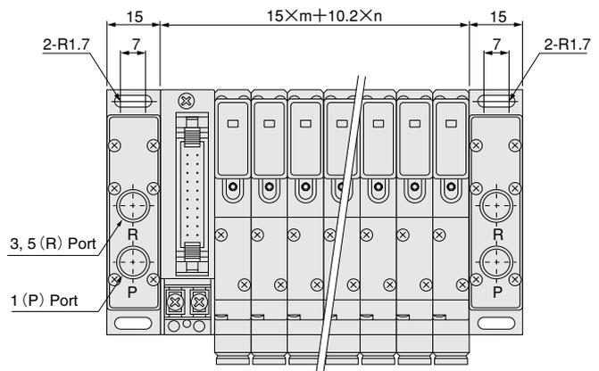
Notes: 1. "m" is the number of wiring modules and piping modules.
