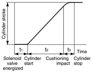
To obtain the time required for the cylinder to complete 1 stroke, add cylinder's delay time  $t_1$  (time between energizing of the solenoid valve and actual starting of the cylinder), to the cylinder's max. speed operating time  $t_2$ . When a cushion is used, add the cushioning time  $t_3$ , to the above calculation. The standard cushioning time  $t_3$  is approximately 0.2 seconds.
