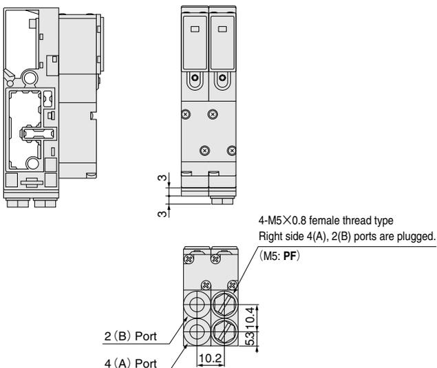
※Height with end block attached is +1mm [0.039in.] longer than indicated below.
