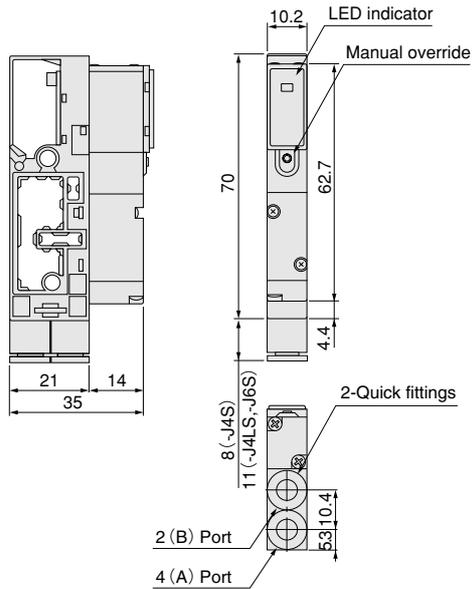
Note: For FMWR090E1, the 2(B) port is plugged, while for FMWR090E1-11, the 4(A) port is plugged ( $\phi$  4: **UP-4**,  $\phi$  6: **UP-6**).
