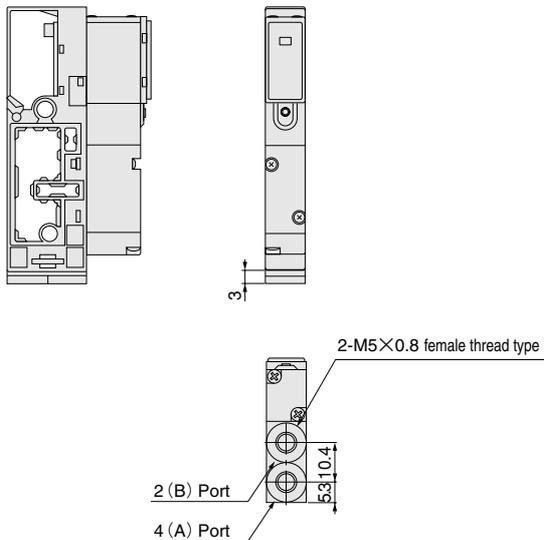
Note: For FMWR090E1, the 2(B) port is plugged, while for FMWR090E1-11, the 4(A) port is plugged (M5: **PF**).
