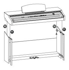
Place the piano body (1) on the frame and attach it with the two hand screws (10) and the two screws M  $6 \times 12$  (11).
