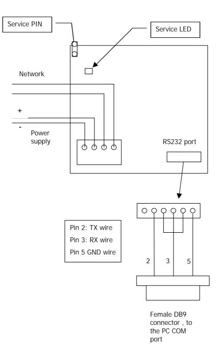
Regarding the power supply connection, please design the power supply line in a way to assure that the node is always powered within the specified operating range.
