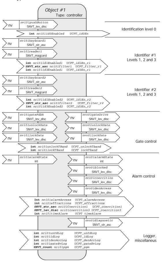
The access controller object is extremely powerful. The LonServer has 8 different access controllers, each one able of handling one access point. An access point is a gate, a door, a barrier or any other device which needs to be activated through an identification process. The identification process can have 4 different levels:
