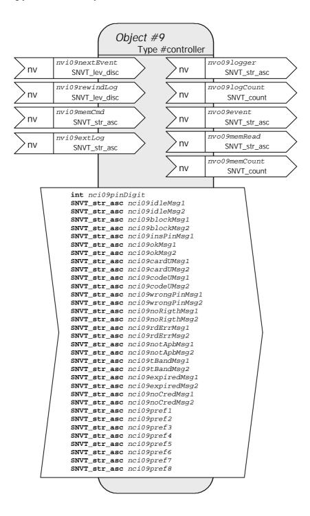
Object 9 contains the network variables to handle the memory information concerning the list of enabled cards, the user types and the logger. This object also stores in several configuration network variables the common access control information, like the user messages, the fixed code, etc.
