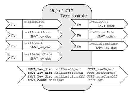
This special controller is used to count people inside a certain area. This kind of controller works in several modes, related to the *nci11pgm* value. At the moment only mode 0 and 1 are enabled. The value 1 is related to card direction detection (see objects 13 and 14 for more details).
