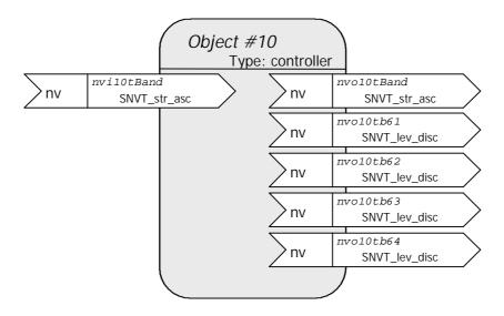
The time band controller handles up to 64 differents weekly time bands. Time bands can be used by all the access control objects. In order to provide general purpose time band outputs, time bands state 61 to 64 are read out using 4 SNVT\_lev\_disc network variables. Each time band has 4 weekly time intervals. When one time interval is active, the whole time band is active as well.
