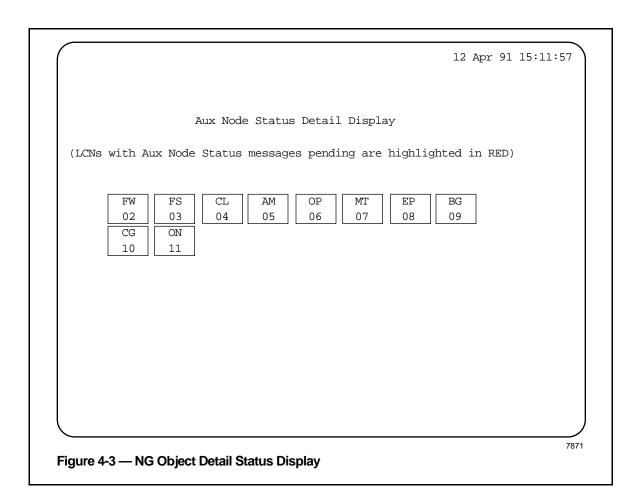
This display shows each of the configured remote systems on this PIN. Each is identified by its System Title and its Local System Number. The box for an individual remote system shows in red if there are any status messages pending that concern that LCN.
