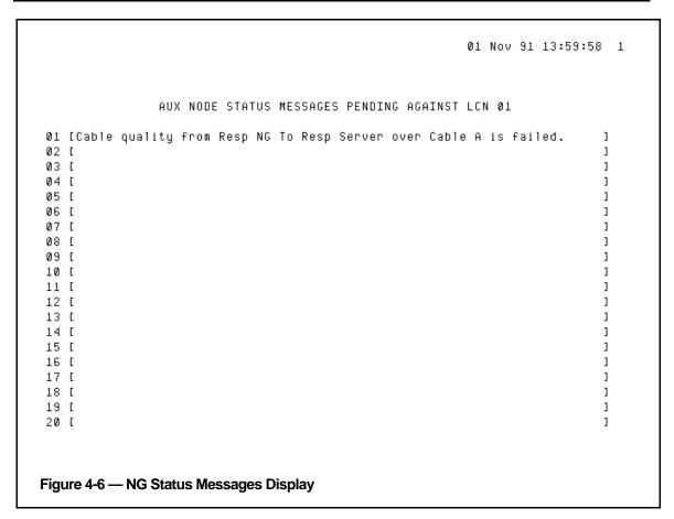
This detail display provides up to 20 current network status messages resulting from configuration or operation errors at the local LCN. Each message is specific to the problem and is intended to be self-explanatory. Each of these messages is due to one of four types of error:
