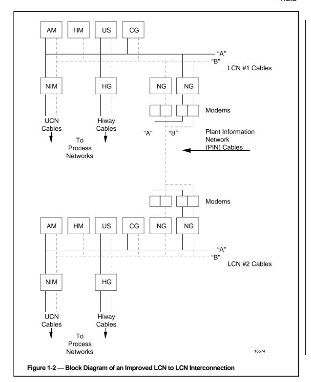
Figure 1-2 shows an improved interconnection that provides alternate routing capability by placing two NGs on each LCN. Note that the NGs are not redundant. Each NG is a separate node (on both the LCN and PIN networks) and software configuration determines what communication traffic runs on each and selects alternate paths for communication. This allows for continued system operation even if one NG should fail.
