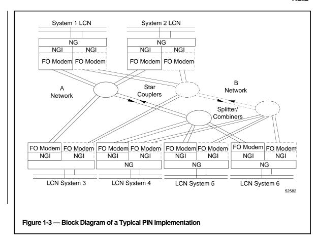
Figure 1-3 shows a broader application of the PIN. It illustrates how more than two LCNs could be interconnected. Note that this example still shows only two NGs on each LCN. The LCN software supports up to 10 NGs per LCN, thus permitting a wide variety of possible communications paths.
