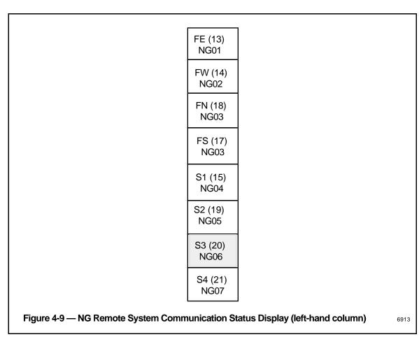
**The left-hand column** of this display shows up to eight of the possible 63 remote systems that could communicate with the local LCN. Each box in this column serves as a header for the 10 by 8 matrix row to its right. Each block of the column shows the "System Name" and the "Local System Number" of a remote system, plus the LCN node address of the local NG that is assigned as the "responsible" communication path to this remote system.
