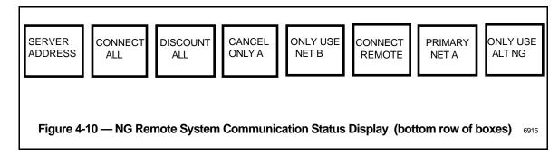
**The bottom row** of boxes provide the targets that cause various actions to occur. Five of the eight boxes always appear although the contents of three of them toggle with use:
