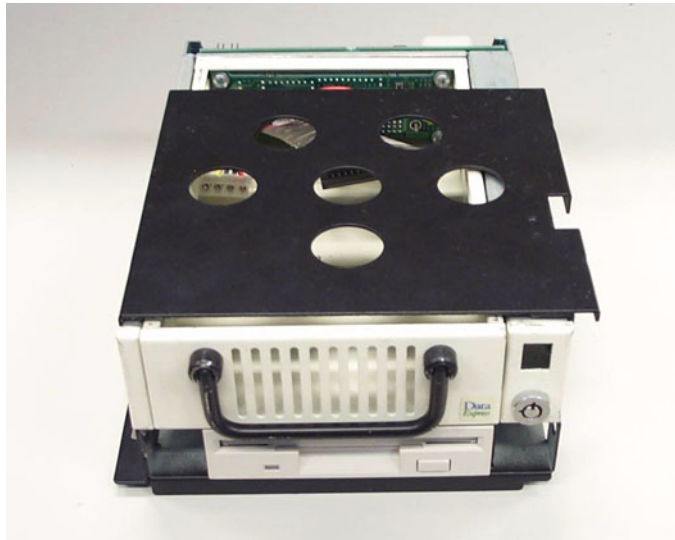
Figure 2.3 Drive bay for 5.25" device and 3.5" FDD
