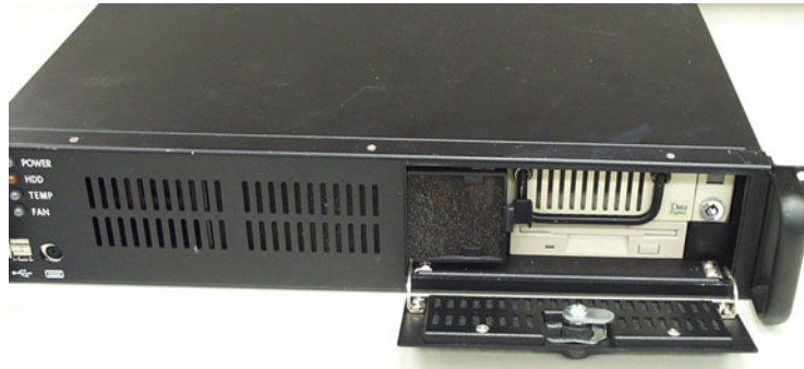
Figure 3.3 Replacing fan filter and door filter
