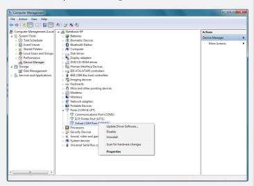
If the 'Virtual COMport' does not install automatically when the USB cable is inserted into the PC, you may need manually update the driver software.
