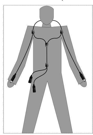
Place the stickman wire over your head and around your neck. Tuck the two male connectors through your jacket sleeve, which you will connect to the heated glove liners.
